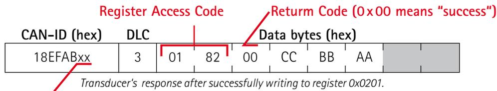
After performing all necessary write accesses, the user might want to save the applied settings to non-volatile EEPROM. Section 9.2.2.1 shows how to do so.
